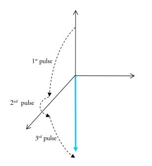
(d.) Note how the middle pulse, which is almost a  $\pi$  pulse, compensates for the missing angle.
