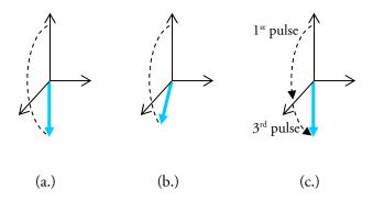
The  $\pi$  pulse in (c.) has no effect because the axis of rotation and the spin's direction are colinear. To appreciate the composite pulse's action, I'm going to enlarge the drawing and exaggerate the angles somewhat:
