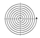
The different trajectories have different advantages. For example, the spiral trajectory above is easier on the gradients. It is also less susceptible to inhomogeneity artifacts (see 2.3 below). It is, however, more tricky to reconstruct the original image because of the irregular sampling (which isn't on a rectilinear grid anymore).
