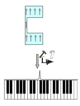
If we were to turn on our z-gradient, we'd be creating a linearly increasing offset. This means the higher up (z-wise) the spins are positioned, the higher the "pitch" they'll emit. Furthermore, loudness of each pitch will be determined by the number of
