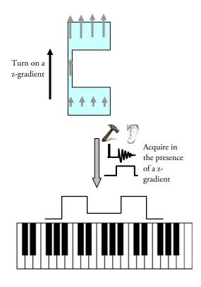
Thus, we "hear" the shape of the sample! That's the idea behind imaging: turn on a gradient, assign a different offset to different positions, excite the sample and "listen". The presence, and intensity, of different frequencies will tell you how many spins (which are proportional to the number of water molecules) you have at each position.
