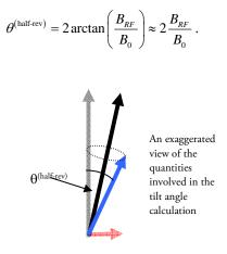
In a full revolution (i.e. in one single oscillation of the RF field), this will get doubled. The number of oscillations the RF will have to complete,  $N_{\text{RF}}$ , is determined by:
