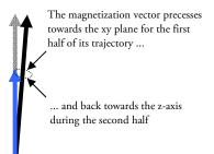
If we reverse the polarity of the RF field midway through after a time  $T^{(rev)}/2$ , we can reverse the direction of the precession and get the spins to keep going towards the xy-plane. We'll have to reverse the polarity again after a time  $T^{(rev)}/2$ , then again after another time  $T^{(rev)}/2$ , and so forth until the spin gets to the xy plane:
