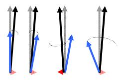
The spin will end up performing a spiral trajectory until it reaches the xy-plane:
