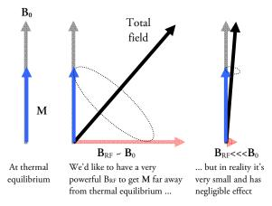
Although in theory even a small tipping will get the spins to precess, the effect will yield a very weak and poor signal. So, can a small RF field tip the spins far away from equilibrium? <u>Yes, if we</u> <u>apply it on resonance</u>. This is the R in NMR.
