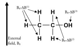
This also means the Larmor frequency of one of the CH<sub>3</sub> protons, for example, is not  $\omega_0=\gamma B_0$  but  $\omega=\gamma B_0-\gamma \Delta B^{(1)}=\omega_0-\omega_{cs}$ . This shift in frequency is termed the chemical shift.
