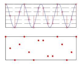
The ADC **discretizes** the signal by sampling it on a regular grid. The horizontal timing between samples,  $\Delta t$ , is called the **dwell time**, and the vertical spacing between samples, is called the **quantization depth** of the ADC.
